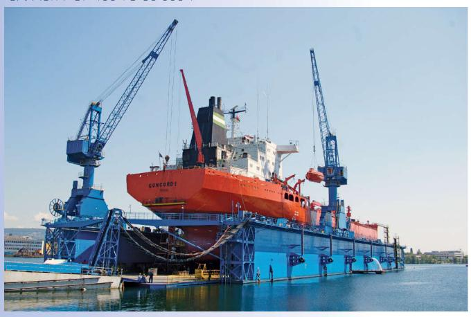
There are the marine constructions designed for shipbuilding and ship repair in sea (ocean) and harbor conditions.
