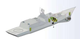
Hydroacoustic stations are designed for detection, position and parameters determination of underwater movable objects, including different small-size objects.
