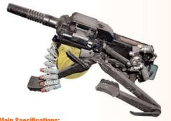
Designed to defeat unprotected enemy's manpower, located on open terrain, behind reverse hill slopes and other similar obstructions, by high-angle and low-angle fire. Highly effective against large-area unprotected targets and concentrated manpower. Mounted on modern combat vehicles and remote weapon stations (RWS), e.g. BMP-1M, BTR-3E1, BTR-4, 'KBA-105TB'1 RWS.
