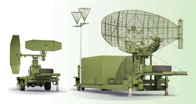
Upgraded Ground-Controlled Approach (GCA) system RSP-10MA is intended to ensure flight safety of aircraft and helicopters within terminal airspace, obtain positional information and guide aircraft to a safe landing in normal and adverse weather conditions. RSP-10MA consists of the surveillance radar (ASR) combining primary and secondary channels and Precision Approach Radar (PAR).
