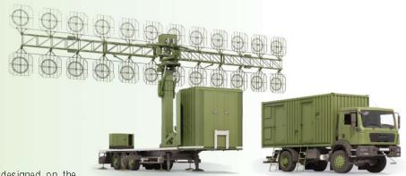
Mobile VHF-band radar AMBER-1800 is designed on the basis of automatically deployed multi-section antenna system. The antenna itself represents a stacked array of dipole-slot antennas with linear horizontal polarization.
