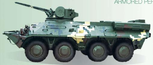
The BTR - 3E1 Armored Personnel Carrier intended to transport mechanized infantry units and to provide fire support in combat operations. It can be used as a basic vehicle forequipping forces quick-reaction marine units. The APC can operate day-and-night, under various climatic conditions, on hard-surface roads, off-road, and in NBC environment.
