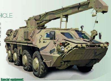
■ crane equipment with lifting capacity of up to 3 t
